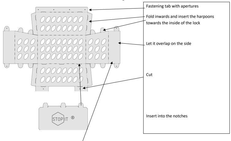
Measure the hive floor and cut out according to the size you have so that the floor of the lock rests on the alighting board
