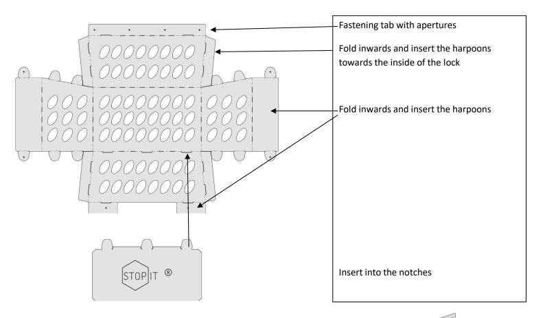
Fasten onto the hive by stapling or screwing on by using the apertures
